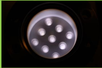
Oxygen plasma during testing of hollow cathode source for the Ultratech Fiji® ALD System conversion.
