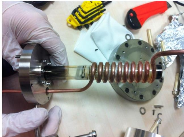
They had previously burnt through the quartz lining of their ICP source. After an ICP replacement, manufacturer recommendations reduced oxygen contamination from ~20% to ~5%, but could not achieve any further reduction.
