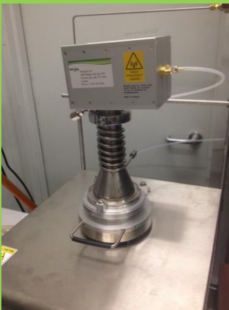
Ultratech Savannah® 100 device conversion used for improved oxide deposition for US government lab.
