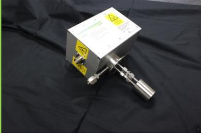
The Meaglow hollow cathode on a NW50 fitting, used for 300 Watt RF operation.
