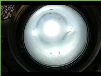
Testing of the hollow cathode plasma source with an oxygen plasma at 100 watts and 300 mTorr.
