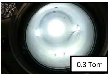
The plasma source to substrate distance is actually not as important as might be thought, as other variables can be changed to greater effect. In particular the gas pressure and flow rate are important.
