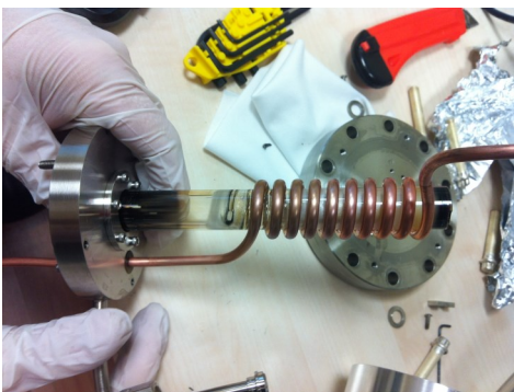
Figure 1: Quartz lining of an ALD system's ICP plasma source, etched through over time.
